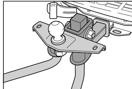
Weight –distributing hitches should be used in many towing conditions. In general, a weight-distributing hitch system is recommended and should be used if you plan to tow trailers with a maximum weight over 5,000 lbs. Refer to trailer and hitch manufacturer for detailed information on load limits. Weight distributing hitches are available in many styles and with sway control accessory options to accommodate trailers with maximum loaded weight and for different driving conditions.
