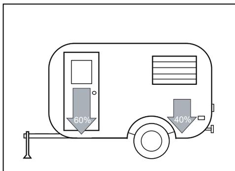
**▲ WARNING-**The trailer load should be balanced equally from side-to-side. Unequal side-to-side loading can negatively affect handling and braking. Once in place, all cargo should be firmly secured to prevent shifting. If the load should shift abruptly during braking or cornering, it could adversely affect the handling and stability of your vehicle and cause a very unsafe situation and may lead to an accident, personal injury or death.
